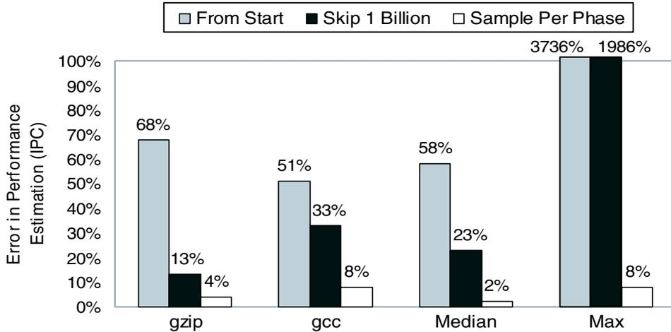
Figure 7: Simulation accuracy for the SPEC 2000 benchmark suite when performing detailed simulation for several hundred million instructions compared to simulating the entire execution of the program. Results are shown for simulating from the start of the program’s execution, for fast-forwarding 1 billion instructions before simulating, and for using SimPoint to choose less than ten 100 million intervals to simulate. The median results are for the complete SPEC 2000 benchmarks.
