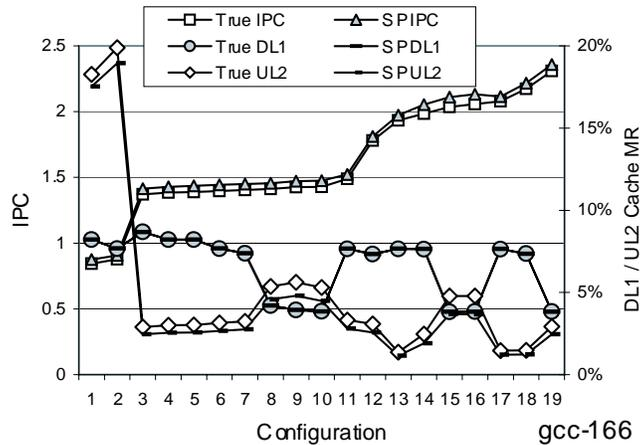
Figure 8: This plot shows the true and estimated IPC and cache miss rates for 19 different architecture configurations for the program `gcc`. The left  $y$ -axis is for the IPC and the right  $y$ -axis is for the cache miss rates for the L1 data cache and unified L2 cache. Results are shown for the complete execution of the configuration and when using SimPoint.
