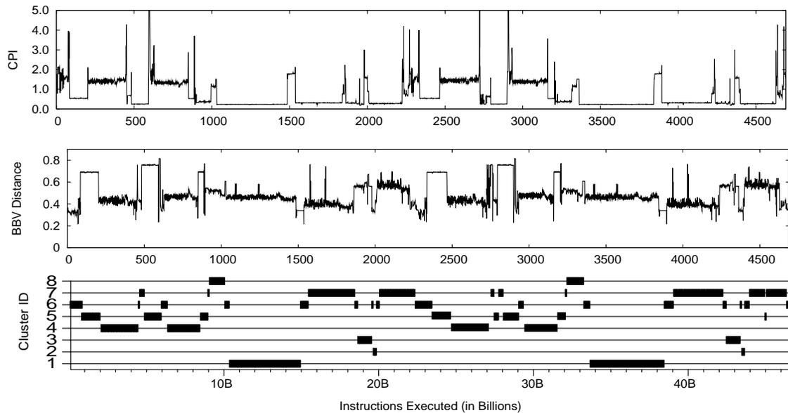
Figure 4: (top graph) Time varying graphs for CPI from each interval of execution for `gcc-166` at 10 million interval size. The  $x$ -axis represents the execution of the program over time. The results are non-accumulative.
