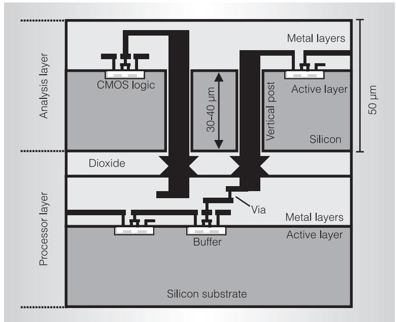
Figure 3. Cross section of the introspective 3D chip, with processor and analysis layers separated by the dioxide layer. The vertical posts are 50 microns in length, with a 5-micron  $\times$  5-micron cross section.
