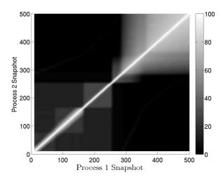
Figure 3: Similarity of cache contents between two instances of *ammp* running with different sets of parameters. The simulations were performed with 1MB direct-mapped cache for first 500 Million references in each execution, which show very high similarity across the diagonal. As we observe regions with high similarity in close vicinity of the diagonal, it can be inferred that the executions own quite similar working sets even if they are not perfectly synchronized.
