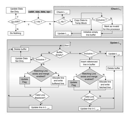
Figure 2: Modifications to cache management technique and cache architecture are indicated as shaded blocks. When a line is evicted from L1 cache, it is merged with pre-existing cache line in L2 if their contents match. We implement exclusive L2 cache as it increases total on-chip memory.
