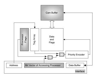
Figure 1: Proposed cache architecture. An array of flags (*processor-flags*) indicates presence of a block for different processors. For *read* operations, processor flag is also checked corresponding to the requesting processor. At *write* operations, lines having same address as the evicted line are brought to CAM and searched for identical content.
