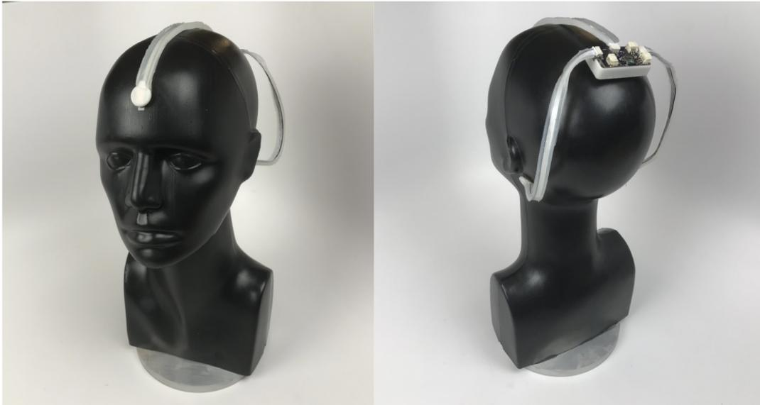
Fig. 5. The MoveU device showing placement of three electrodes, two on the mastoids and one on the forehead. Electrode placement along with current intensity, direction and duration determines the sensation felt.
