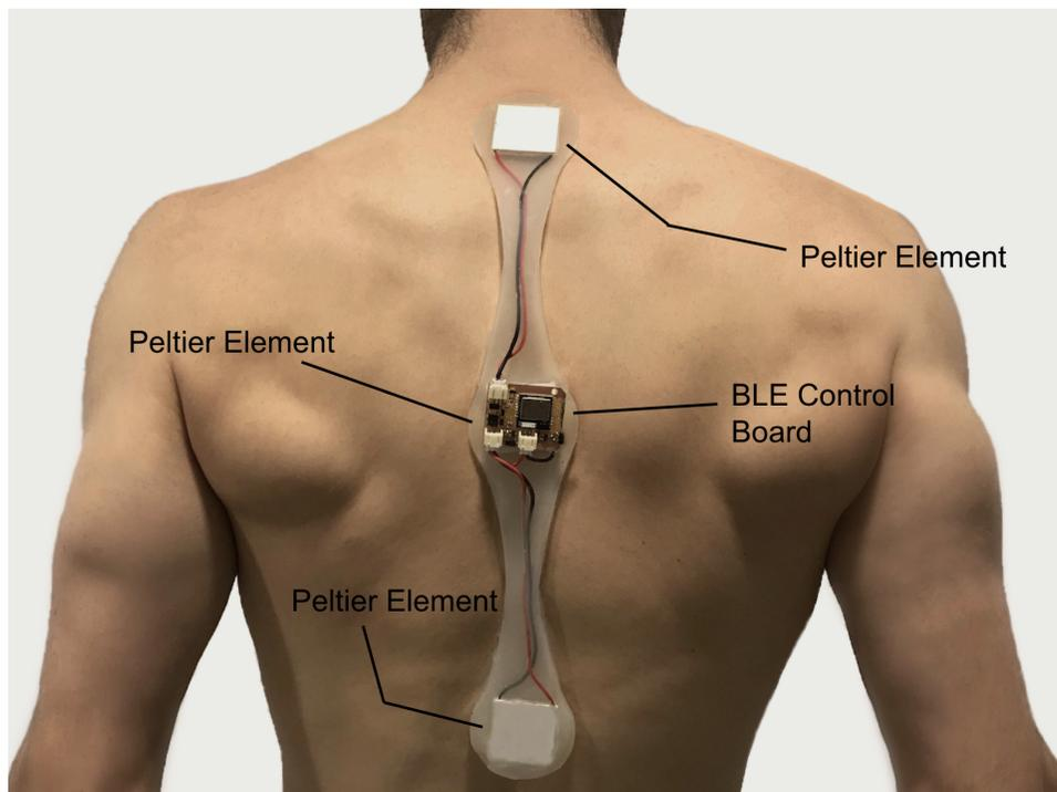
Fig. 7. Frisson wearable device showing the Peltier elements and their placement on the back to elicit aesthetic chills.
