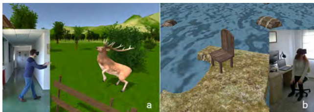
Figure 2: Examples of user interaction in the virtual world. (a) Proximity based interaction with virtual elements (virtual world as seen from a first person perspective). (b) Interaction with a real chair through passive haptics (virtual world as seen from a third person perspective).
