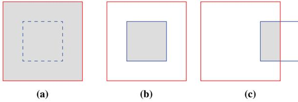
Figure 2: The three physical space to shared virtual space mapping techniques we designed: (a) Scale, (b) Kernel, and (c) Overlap. The red outline shows the larger physical space ( $L$ ) and the blue outline shows the smaller physical space ( $S$ ). Shared virtual space is shown in gray.
