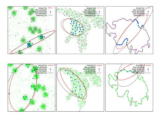
Fig. 6. The figure shows detection of ellipse-shaped events on three different data sets: clustered, Lake, and Temperature. The maximum estimation error in these examples is again less than 0.01n for the first row (140 monitors). By decreasing the number of monitors to 50, we find that in some cases the estimation error increases, we have shown the representative examples for these cases in the second row.
