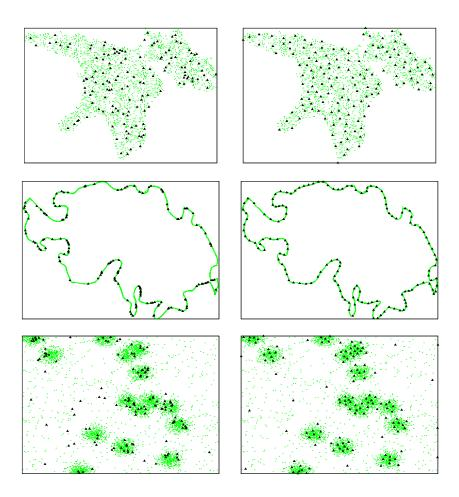
Fig. 4. Regular random sampling (left), and REDUNDANCY-AWARE sampling (right) with equal number of monitors. First row shows the results for Lake dataset, the second one for Contour dataset and the third row shows the results for Clustered Dataset.
