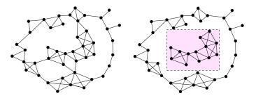
Fig. 1. The figure shows that the global connectivity can change substantially without any significant change in the local connectivity of the nodes: the loss of just a few isolated edges can cause major network partitions.
