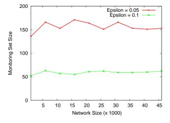
Fig. 8. The monitoring set sizes for  $\varepsilon=0.05$  and 0.10 for different network sizes.
