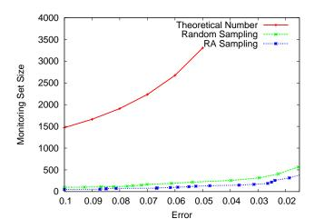
Fig. 3. The size of the monitoring set for various values of the parameter  $\varepsilon$ . The top curve is the theoretical bound; the second curve is computed by empirical data. The third curve shows the improvement given by Redundancy-Aware sampling, which is described in the next subsection.
