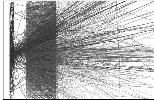
Fig. 21. SPL - genetic algorithm with bezier lines. The chromosomes are characterized by a set of x coordinates, a slope and a intercept. the y coordinates will be calculated using the line function y = m \cdot x + b (where m = slope and b = intercept) Each line then acts as Bezier handles, for shaping the curve. Each "generation" is a single curvy contour with multiple Bezier handles (the lines) in between.
