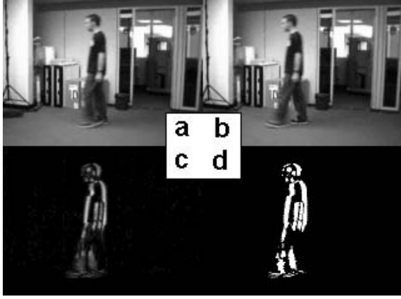
Fig. 2. Temporal Differencing Example. a) Previous Frame b) Current Frame c) Difference (normalized for display purposes) d) Thresholded Difference
