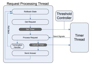
Figure 4: Request execution flow with SERT.
