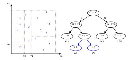
Once again, find a split variable and a split value that minimize the predicted error, here  $x_2$  and  $v_4$ .
