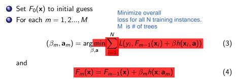
For each iteration, we only determine one tree classifor h(). How to minimize loss for one tree? Try to find a function close to residual yi-F
