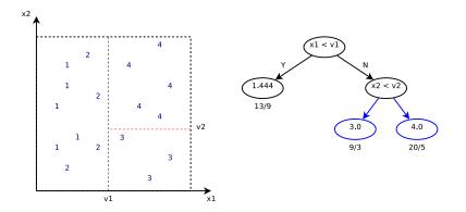
Here we examine the right side first: find a split variable and a split value that minimize the predicted error, i.e.  $x_2$  and  $v_2$ .
