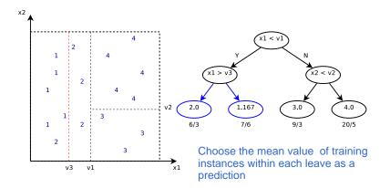
Now to the left side: Again, find a split variable and a split value that minimize the predicted error, i.e.  $x_1$  and  $v_3$ .
