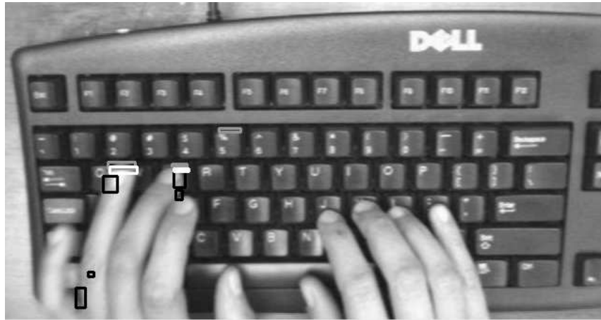
(a) Hand tracking analysis. Rectangles identify regions in movement. Black rectangles are used for movements in the hands regions, grey rectangles for keys, white rectangles for regions where both hand and key movement happens. These rectangles identify likely key pressings.
