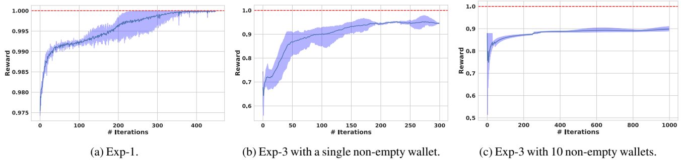
Figure 4: The agent’s normalized reward in Exp-1 and Exp-3. The x-axis is the training iteration, and y-axis is the normalized reward. The solid lines are the average, and the lighter bands indicate the variations between the maximal and minimal reward.
