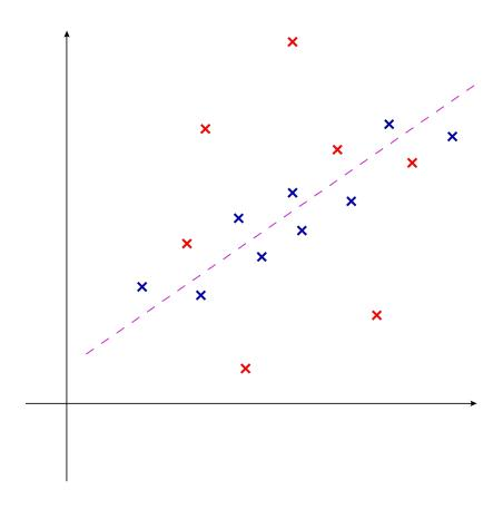
Find the two points that resulted in the smallest median error. Pick half of the points with the smallest error. Recompute the line as a least-squares fit with this set of points.
