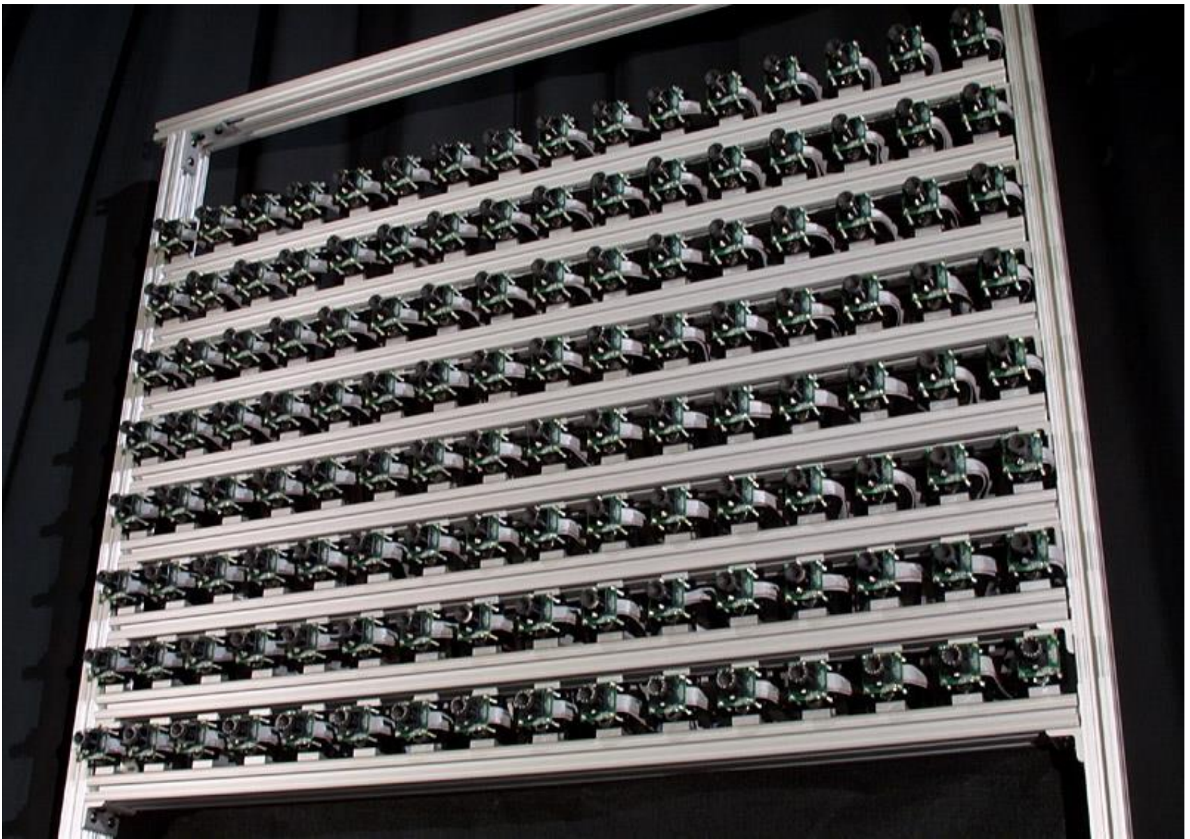
The Stanford Multi-Camera Array 128 CMOS cameras, 2" baseline
