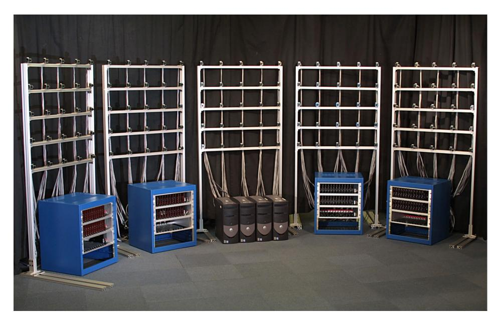
**5x5 racks version:** 125 CMOS cameras, 9" baseline 4 capture PCs, 4 electronics racks (1 board per camer
