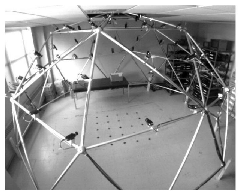
**CMU multi-camera stereo** 51 video cameras mounted on a 5-meter diameter geodes
