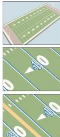
THE VIRTUAL FIELD The computer-generated map of the field appears as a blue grid on the computers used. It is manipulated to fit the cameras' views.
