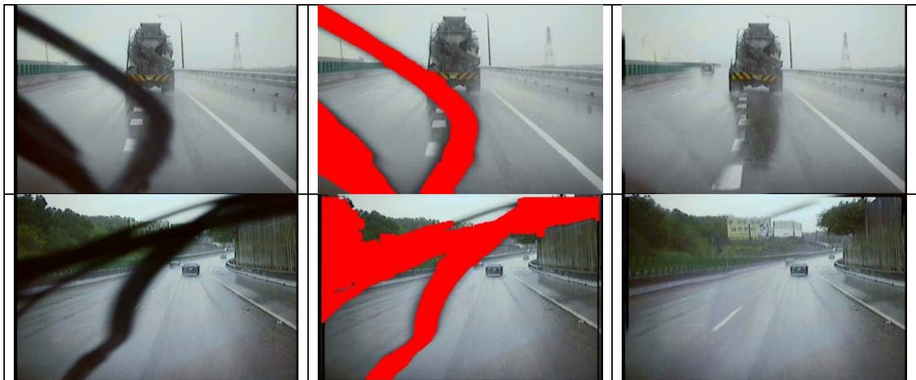
Figure 1 (a) a video frame with the wiper presence, (b) the wiper frame with the wiper detected and localized automatically by our computer program (wiper pixels are marked in red), and (c) wiper pixels in the wiper frame are replaced by the corresponding pixels in the adjacent non-wiper frame to provide better viewing of the surrounding.
