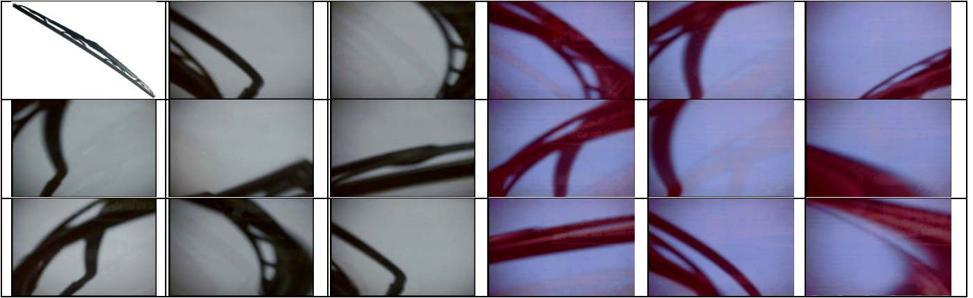
Figure 2 Upper-left corner: a standard "coat-hanger" wiper, and the rest: different ways a standard wiper can appear in an onboard video (the pictures were taken against a uniform background for clarity).
