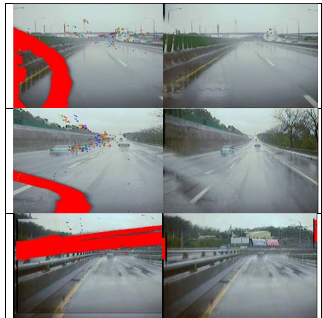
Figure 4 Sample results of wiper region detection and localization (left) and in-painting (right)
