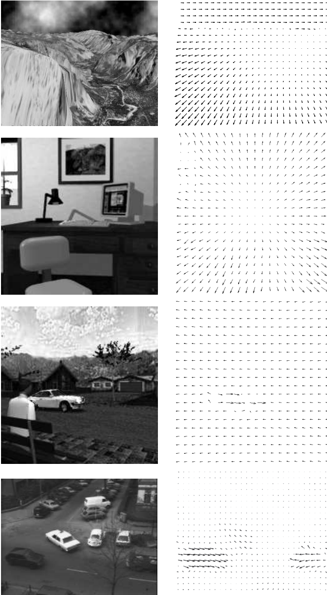
Figure 4. Left: a sample frame in the video sequence. Right: the computed optical-flow field. From top to bottom: Yosemite, Office, Street, and Taxi sequences.
