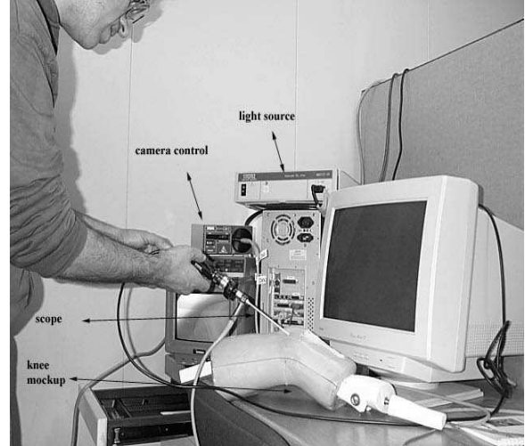
Fig. 3. Experiment platform of a knee mockup, a camera and control, a scope, and a light source.
