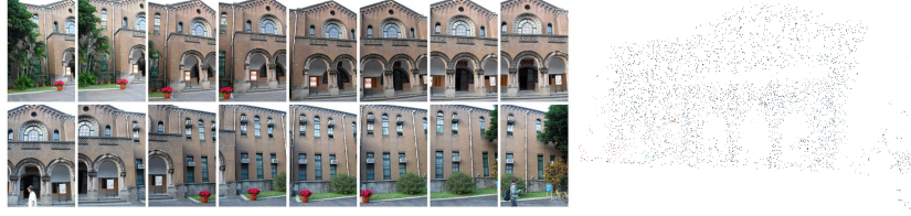
Fig. 1. An example of MVS data. Left: input images; right: output point clouds.
