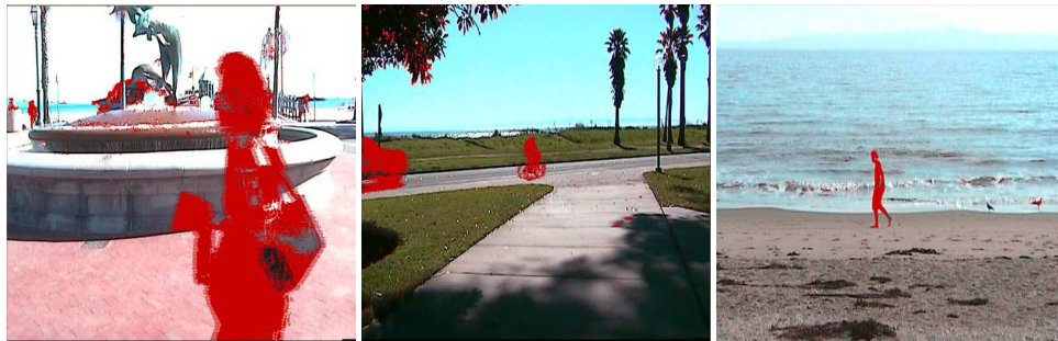
Figure 7: Sample foreground/background identification results. Pixels marked red are identified as foreground pixels. Even though large color changes due to wave, water, and vegetation movements are observed in these pictures, the algorithm correctly eliminates background motion from consideration.
