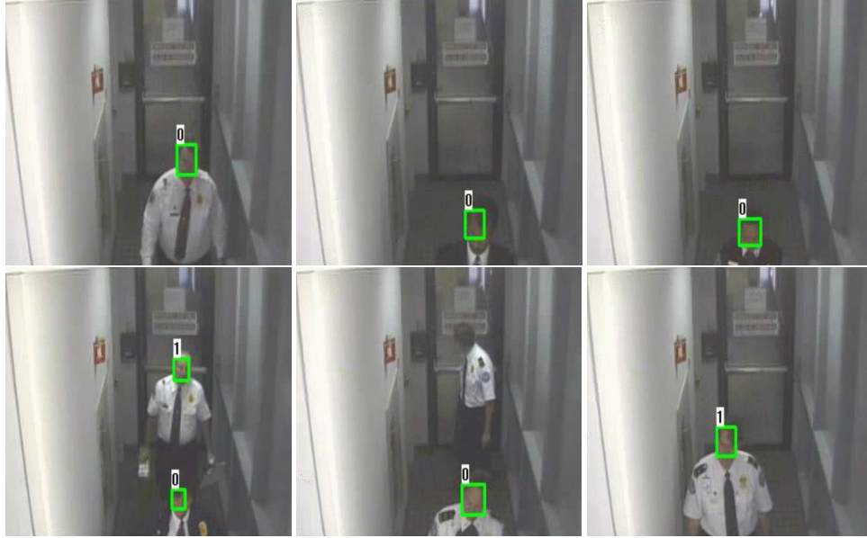
Figure 3: Sample results of detecting unauthorized piggy-backing access patterns. In the top row, three legal single person entrance scenarios are shown. In the bottom row, two piggy-backing access patterns are shown. The image on the bottom left shows two face regions detected in a single frame. The two images on the bottom right show two face regions detected in different video frames within a short time interval to trigger piggybacking alarm (the two face regions are marked as 0 and 1, respectively.)
