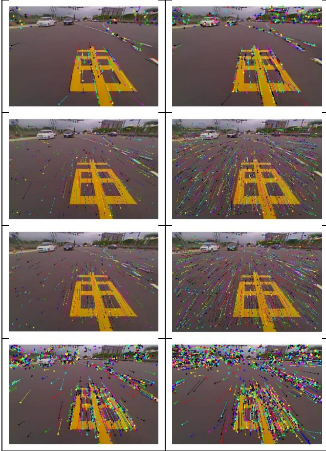
Figure 10 Sample baseline + regularization + median filter + magnitude threshold tracking results. Left column: the paring margin set at 0.7 (tightest) and right column: the paring margin set at 0.95 (loosest). From top to bottom: SIFT, SURF, USURF and ZBRIEF. These figures are in one-to-one correspondence with those in Figure 6 to show the enhancement using our analysis.
