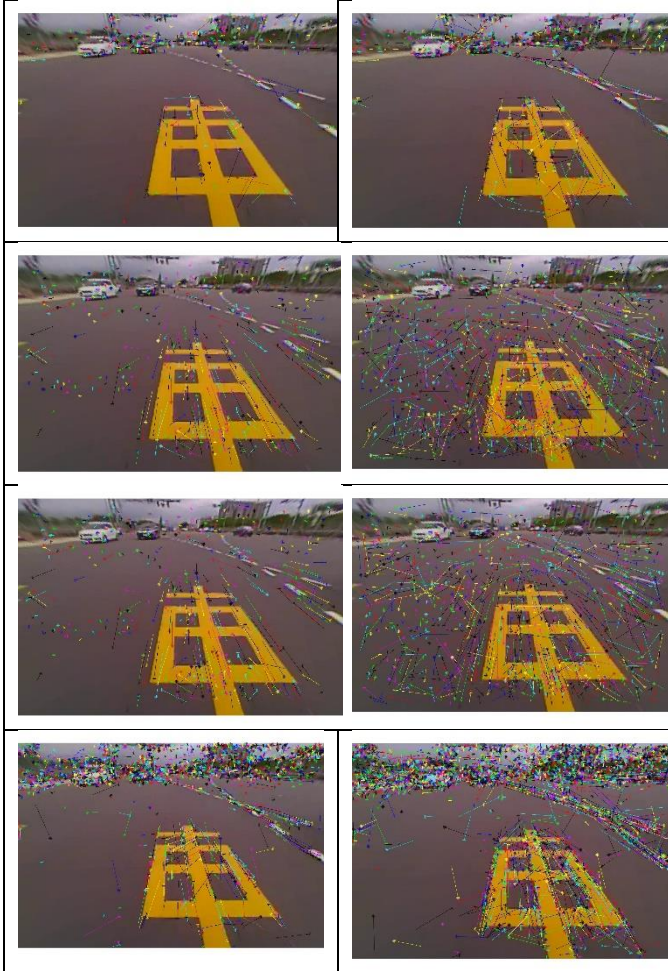
Figure 6 Sample baseline tracking results. Left column: the pairing margin set at 0.7 (tightest) and right column: the pairing margin set at 0.95 (loosest). From top to bottom: SIFT, SURF, USURF and ZBRIEF.
