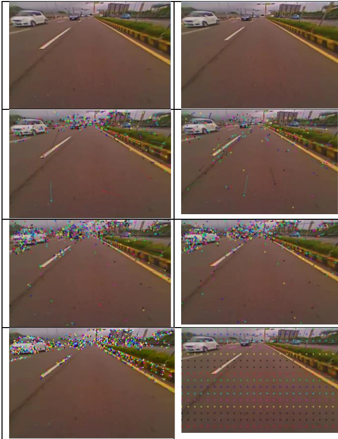
Figure 2 Sample results of applying standard trackers to distortion corrected images. First row: two input frames for tracking, second row: accurate feature-based trackers (left: SIFT, right: SURF), third row: efficient feature-based trackers (left: BRIEF, right: ZBRIEF), and last row: flow-based trackers: (left: KLT, right: dense optical flow).
