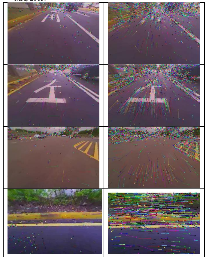
Figure 11 More sample results using ZBRIEF. Left: with a tight margin and without any enhancement and right: with a loose margin and with all enhancements. First two rows are from a front-mounted camera with a zoom-out flow, 3rd row is from a back-mounted camera with a zoom-in flow and last row is from a side-mounted camera for a translational flow.
